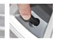
Inspect whether there is any damage or crack caused by installation on the valve surface.
