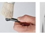
Lubricate the Snap-in valve with soap water or a mounting paste to decrease the friction between valve and rim hole, avoiding the valves surface damage.
